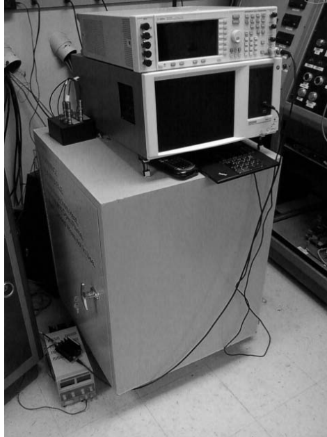
Figure 16. Measurement equipment located in the control room. On the floor (left), DC power supply with RF amplifier resting on top. On the workbench (bottom) the Keithley 4200 with signal generator on top. A signal control box (sitting to the left of the 4200) was designed to pass signals to and from the 4200 onto the CAT 5 cable.
